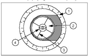
**Fig. 6:** Correct Collimation. (1) Round Edge of Focuser Drawtube; 2) Secondary Mirror; (3) Spider Vanes; (4) Eye.
